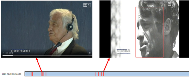
Fig. 6. Example of the output of the TV personality recogniser. The video timeline is synchronised and annotated with the names of the identified TV personalities.
