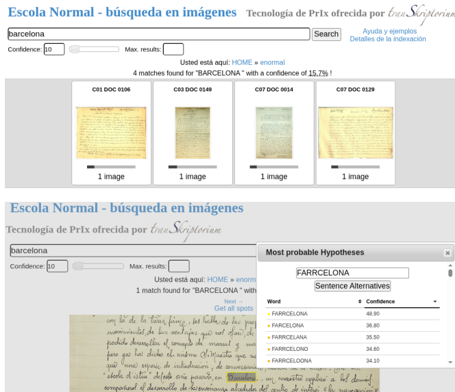
Fig. 1. Example of the search system when looking for the word “barcelona”. The top image shows the four retrieved images when the confidence threshold is set down to 10%. The bottom image shows possible word hypotheses and the corresponding relevance score for the top-ranked words.
